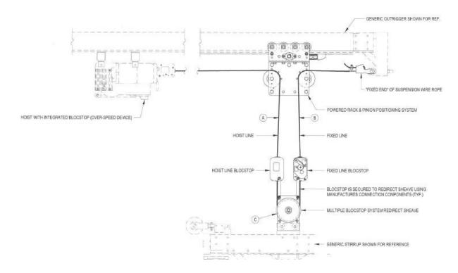
8. The diagram in the preceding paragraph depicts the following configuration for a single suspension wire rope on the swing stage scaffold (the described routing is from left to right on the diagram): from an electrically powered winding device located on the outrigger (not
