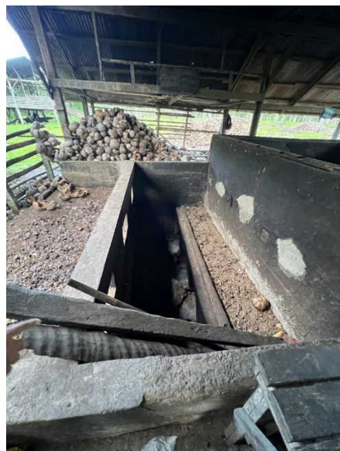
Traditional smoke kiln fueled by coconut shells, used in processing coconuts into copra on the farm
