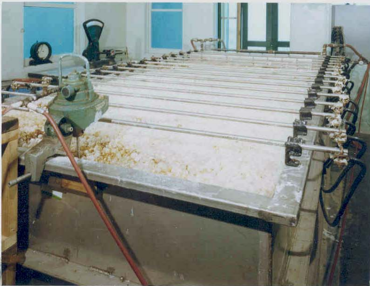
TOP LEFT - 25 LB. LEAD AZIDE DISSOLVING IN \text{NaOH} . TOP RIGHT - \text{NaOH} CIRCULATING SYSTEM. BOTTOM LEFT - 2000 GALLON PLATING TANK. BOTTOM RIGHT - PLATING ELECTRODES.
